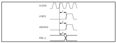
Figure 66 Timing of the IMA Interface
