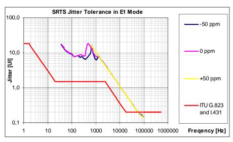
Figure 43 SRTS Jitter Tolerance in E1 Mode without Jitter Attenuator
