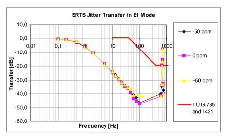
Figure 51 SRTS Jitter Transfer in E1 Mode without Jitter Attenuator
