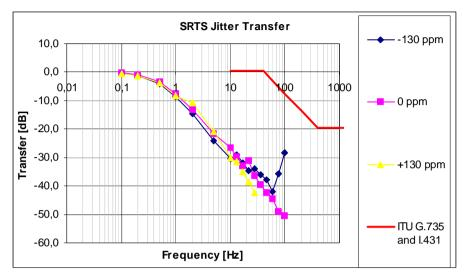
Figure 53 SRTS Jitter Transfer in T1 Mode without Jitter Attenuator
