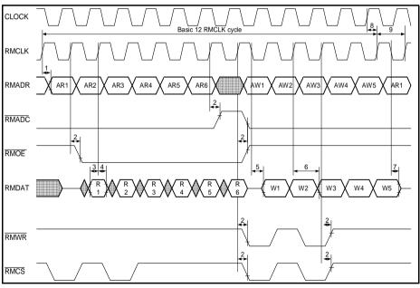
Figure 71 RAM Interface Timing Diagram
