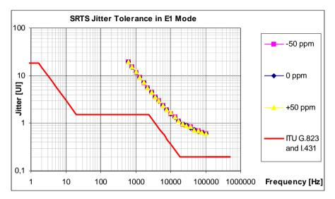
Figure 44 SRTS Jitter Tolerance in E1 Mode with Jitter Attenuator
