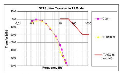
Figure 54 SRTS Jitter Transfer in T1 Mode with Jitter Attenuator
