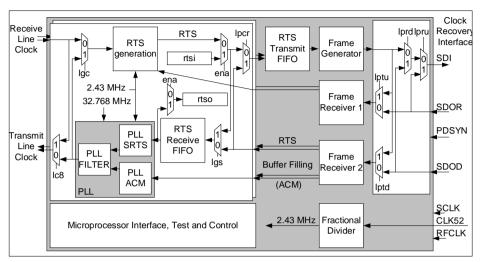
Figure 19 Block Diagram of the ICRC
