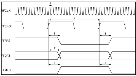
Figure 60 Framer Transmit Interface Timing in GIM
