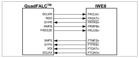
Figure 22 Connection of IWE8 to QuadFALC
