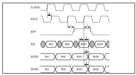
Figure 67 Clock Recovery Interface Timing Diagram
