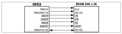
Figure 34 External RAM Connection
