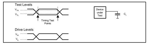
Figure 55 Input/Output Waveforms for AC Measurements
