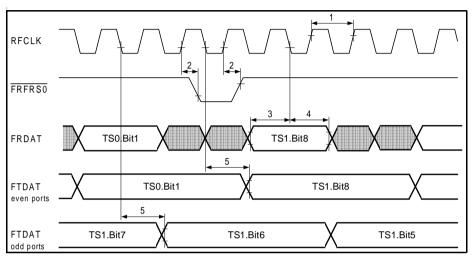
Figure 63 Framer Interface Timing in EC Mode
