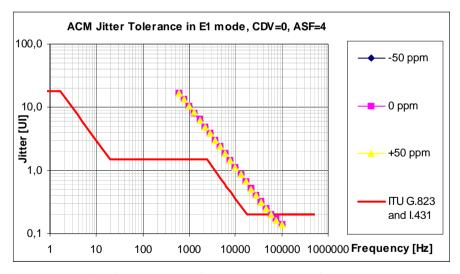
Figure 39 ACM Jitter Tolerance in E1 Mode without Jitter Attenuator
