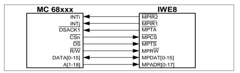
Figure 33 Connection of IWE8 to an Motorola Type Microprocessor
