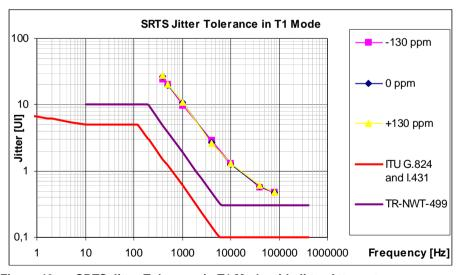
Figure 46 SRTS Jitter Tolerance in T1 Mode with Jitter Attenuator
