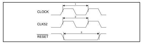
Figure 56 Clock and Reset Interface Timing Diagram
