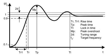
Figure 20 Transient Parameters
