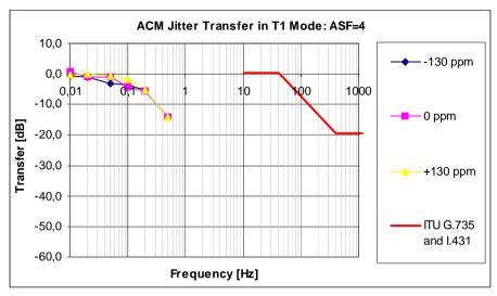
Figure 49 ACM Jitter Transfer in T1 Mode without Jitter Attenuator
