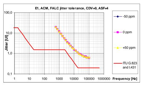
Figure 40 ACM Jitter Tolerance in E1 Mode with Jitter Attenuator
