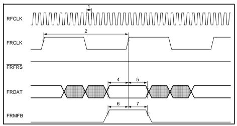
Figure 59 Framer Receive Interface Timing in GIM
