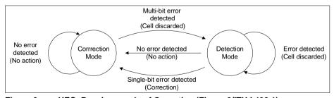
Figure 9 HEC: Receiver mode of Operation (Figure 3/ITU I.432.1)
