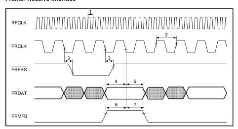
Figure 57 Framer Receive Interface Timing in FAM
