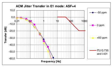
Figure 47 ACM Jitter Transfer in E1 Mode without Jitter Attenuator
