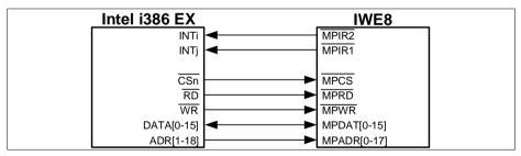
Figure 32 Connection of IWE8 to an Intel Type Microprocessor
