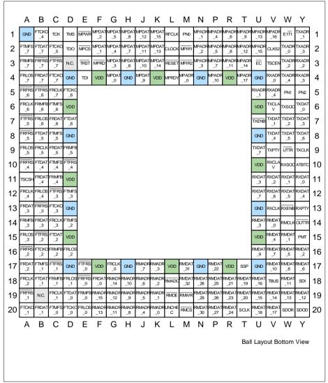
Figure 5 Pin Configuration
