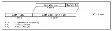
Figure 13 SAR-PDU of AAL Type 0
