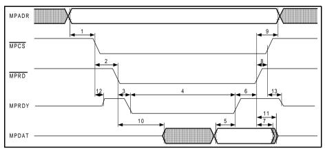
Figure 69 Intel Mode Read Cycle Timing Diagram
