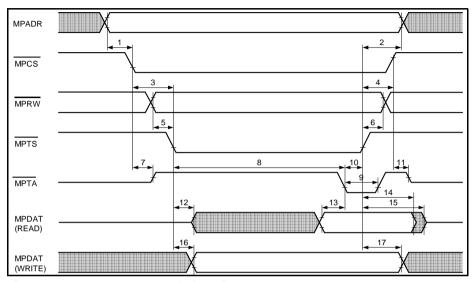
Figure 70 Motorola Mode Timing Diagram
