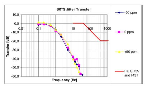
Figure 52 SRTS Jitter Transfer in E1 Mode with Jitter Attenuator
