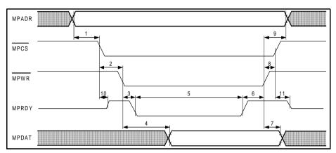
Figure 68 Intel Mode Write Cycle Timing Diagram
