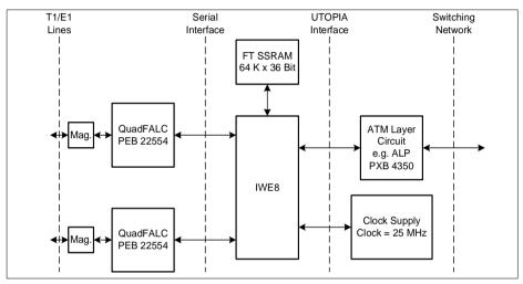
Figure 3 Line Card for 8 T1/E1 Channels
