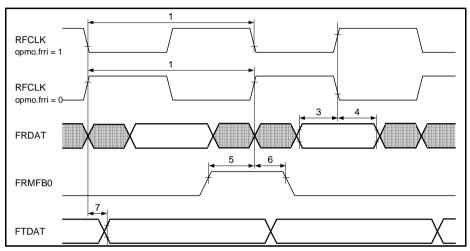
Figure 61 Framer Interface Timing for SYM 2.048 MHz
