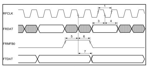
Figure 62 Framer Interface Timing in SYM 8.192 MHz
