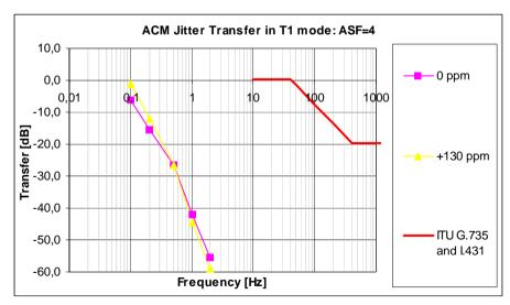
Figure 50 ACM Jitter Transfer in T1 Mode with Jitter Attenuator
