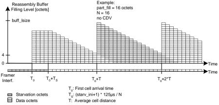
Figure 15 Reassembly Buffer Initialization: No CDV
