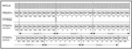
Figure 28 Framer Interface in EC Mode
