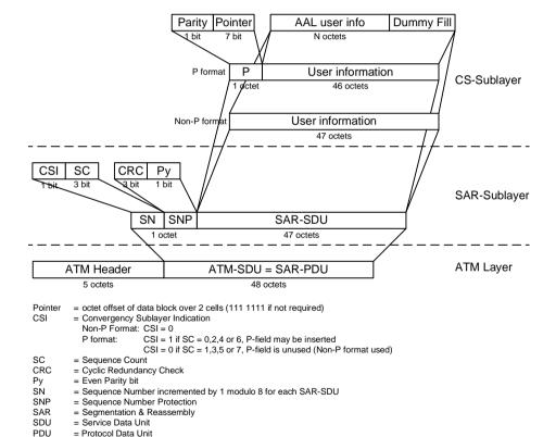
Figure 74 Structure of the AAL1 SAR-PDU
