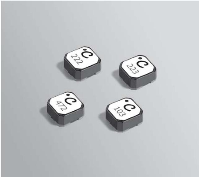
At only 1.4 mm high and 3 mm square, the LPD3015 is Coilcraft's smallest shielded coupled inductor. The excellent coupling coefficient ( $k \geq 0.97$ ) makes it ideal for use in SEPIC applications. In SEPIC topologies, the required inductance for each winding in a coupled inductor is half the value needed for two separate inductors, allowing selection of a part with lower DCR and higher current handling.
