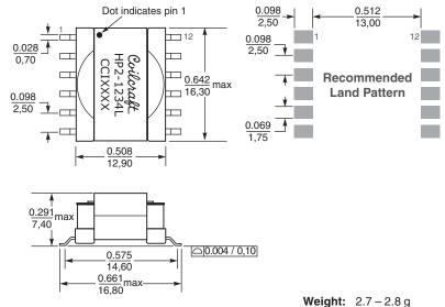
Dimensions are in  $\frac{\text{inches}}{\text{mm}}$
