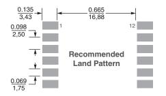
Weight: 4.2 – 4.6 g Packaging 200 per 13" reel Plastic tape: 44 mm wide, 0.4 mm thick, 28 mm pocket spacing, 9.6 mm pocket depth
