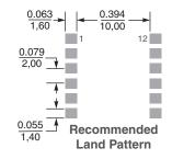
Weight: 1.4 g Packaging 500 per 13" reel Plastic tape: 24 mm wide, 0.5 mm thick, 20 mm pocket spacing, 6.6 mm pocket depth
