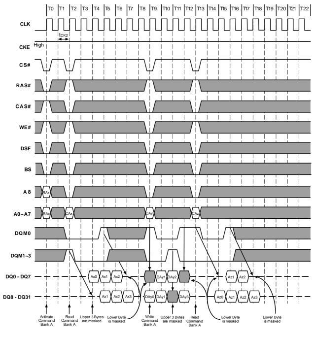
Figure 20. Byte Write Operation (Burst Length=4, CAS# Latency=2)
