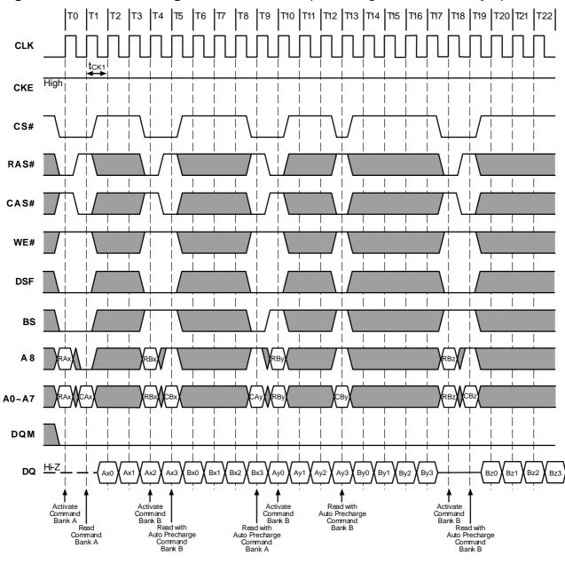
Figure 16.1. Auto Precharge after Read Burst (Burst Length=4, CAS# Latency=1)
