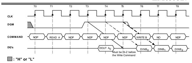
Read to Write Interval (Burst Length; Ù 4, CAS# Latency = 3)
