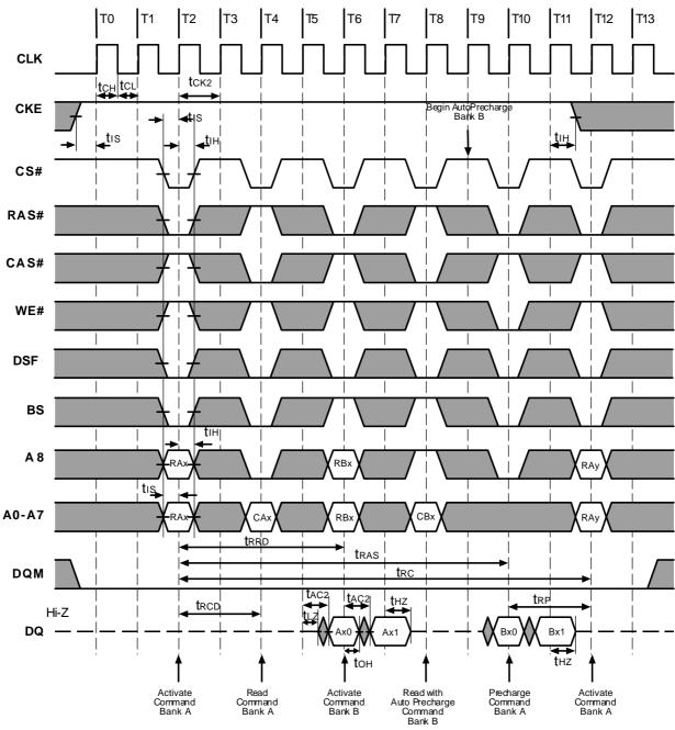
Figure 2. AC Parameters for Read Timing (Burst Length=2, CAS# Latency=2)
