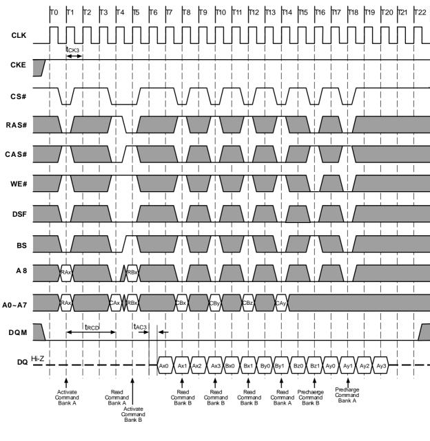
Figure 14.3. Interleaved Column Read Cycle (Burst Length=4, CAS# Latency=3)
