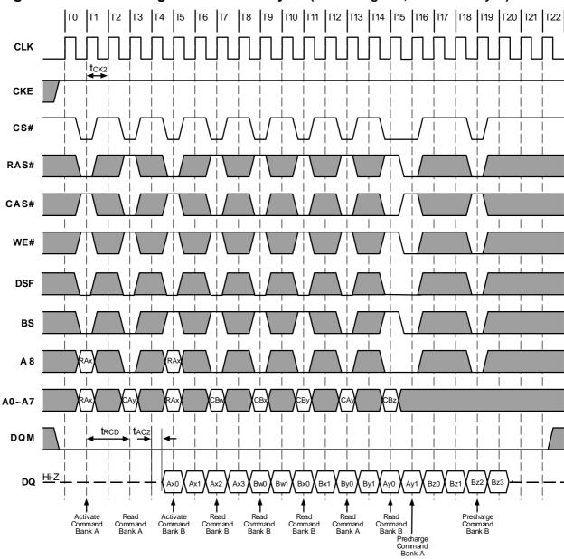
Figure 14.2. Interleaving Column Read Cycle (Burst Length=4, CAS# Latency=2)
