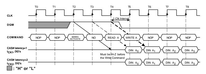
Read to Write Interval (Burst Length; Ù 4, CAS# Latency = 1, 2)
