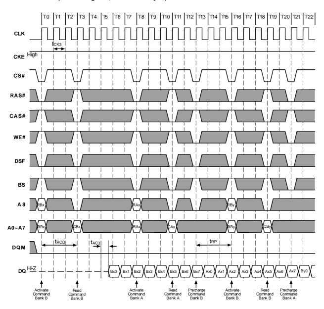
Figure 12.1. Random Row Write (Interleaving Banks)
