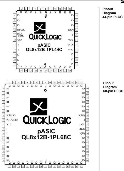
Pins identified I/SCLK, SM, SO and SI are used during scan path testing operation.
