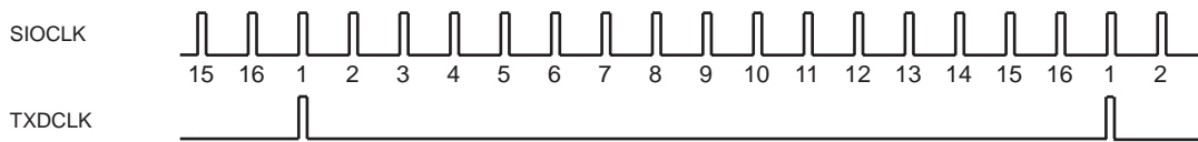
Figure 7-3 Generation of the Transmission Clock
