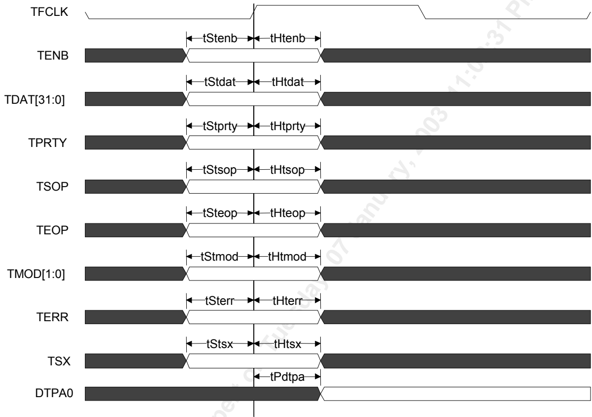
Figure 30 POS-PHY Level 3 Transmit Physical Timing
