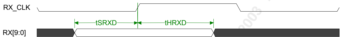
Figure 33 TBI Receive Physical Timing
