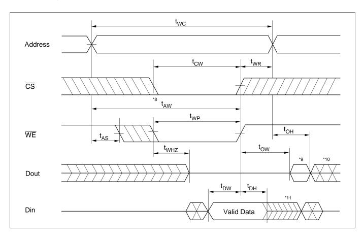
Write Timing Waveform (2) (OE Low Fixed)
