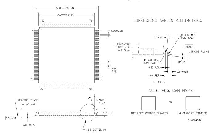
100-Pin Thin Plastic Quad Flat Pack (TQFP) A100
