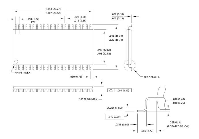
**NOTE:** 1. All dimensions in inches (millimeters) <u>MAX</u> or typical where noted.
