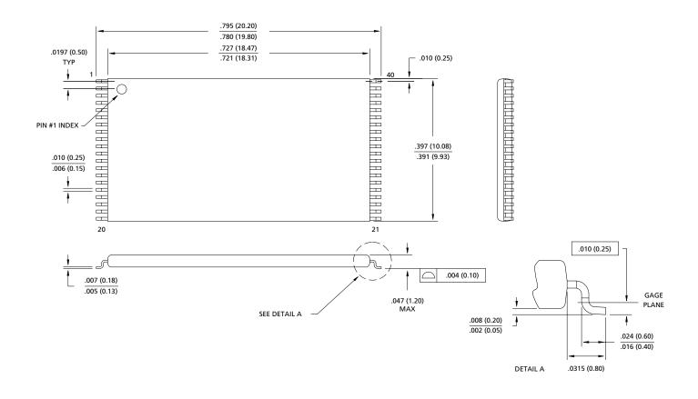
**NOTE:** 1. All dimensions in inches (millimeters)  $\frac{MAX}{MIN}$  or typical where noted.
