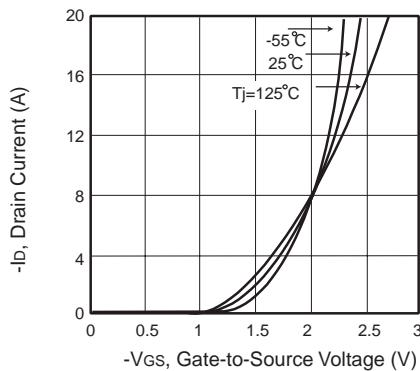
Figure 2. Transfer Characteristics
