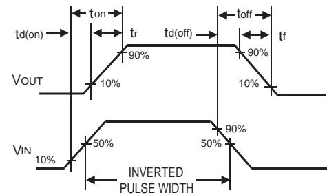
Figure 12. Switching Waveforms
