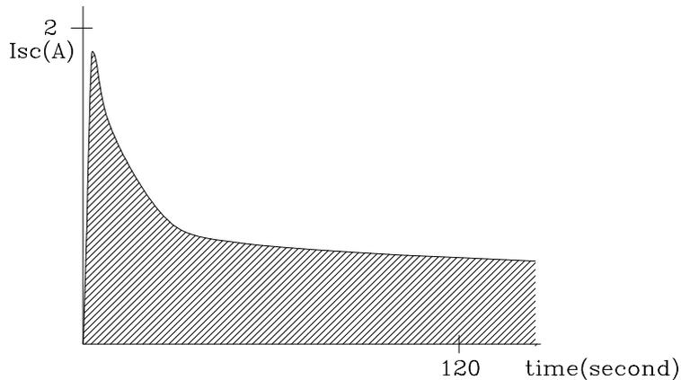
As the territory of the deviant line appear by the heat, as the area is wider,  $T$ (The PCB substrate temperature in 2 minute) is becoming high.
