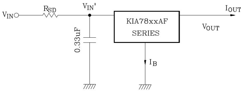
The power dissipation  $P_D$  of IC is expressed in the following equation.
