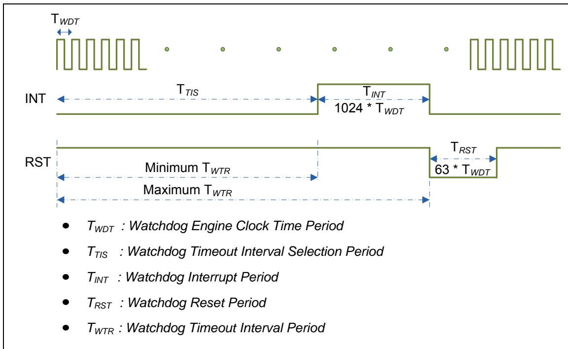
Figure 5-11 Timing of Interrupt and Reset Signal
