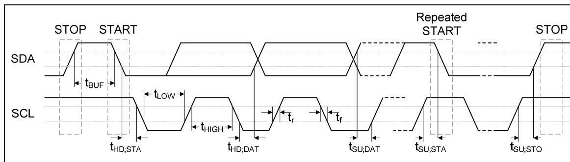
Figure 5-10 I<sup>2</sup>C Bus Timing
