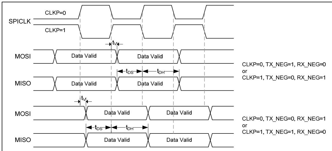
Figure 7.5-1 SPI Master dynamic characteristics timing
