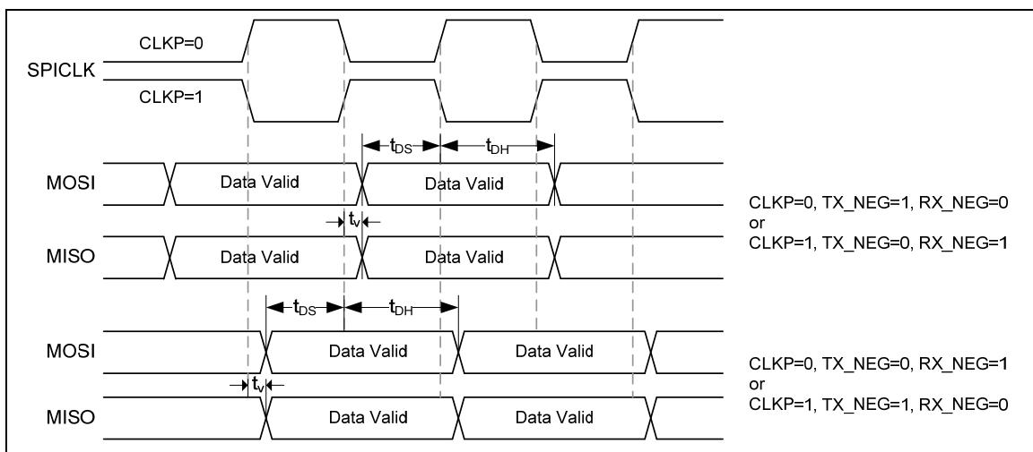
Figure 7.5-2 SPI Slave dynamic characteristics timing
