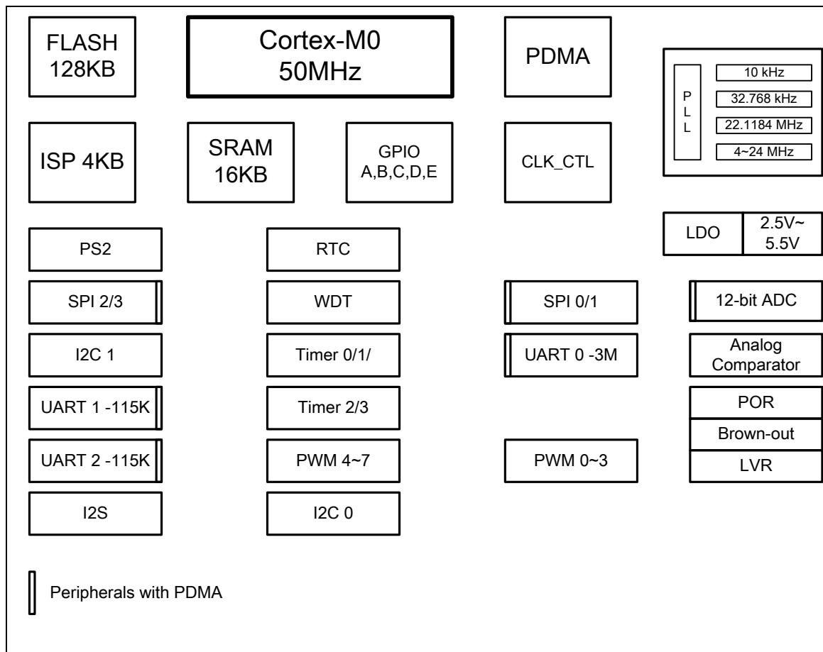
Figure 4-1 NuMicro™ NUC100 Medium Density Block Diagram
