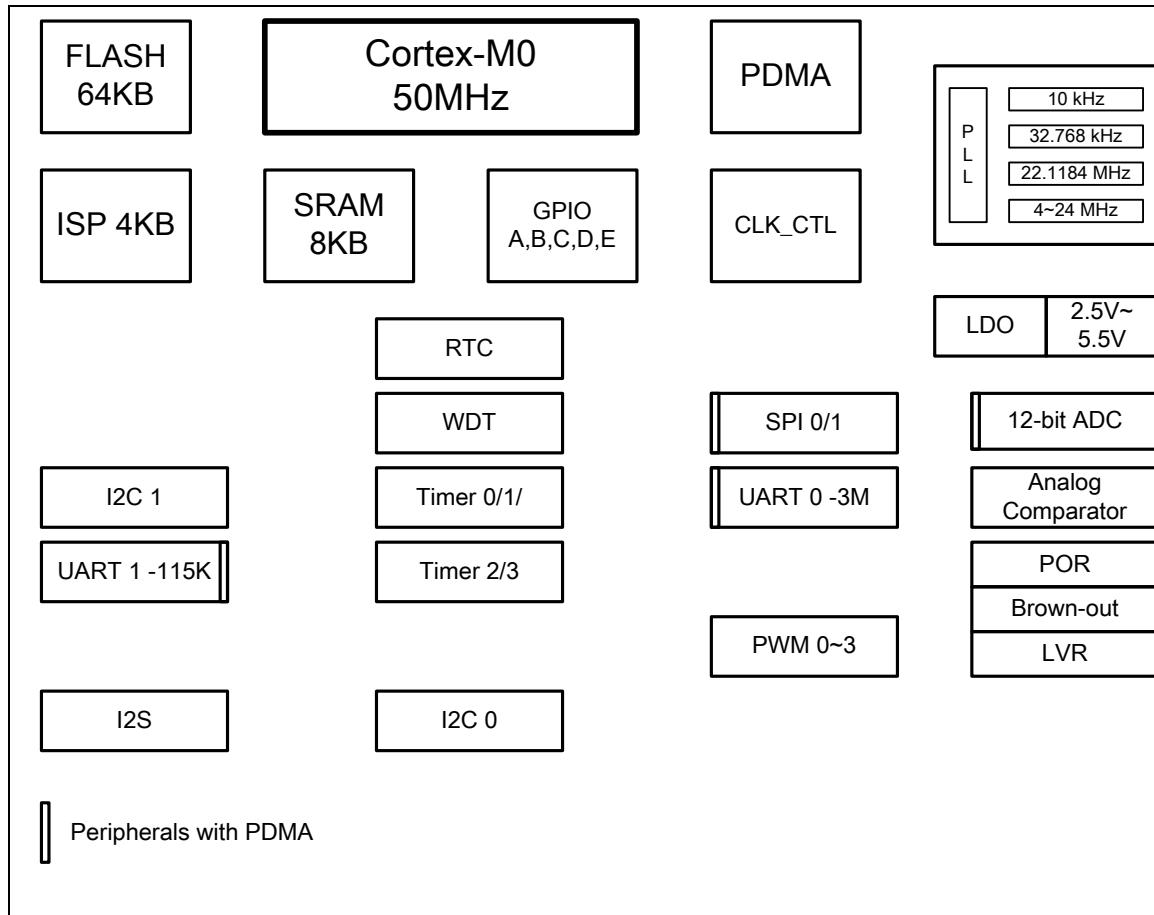
Figure 4-2 NuMicro™ NUC100 Low Density Block Diagram
