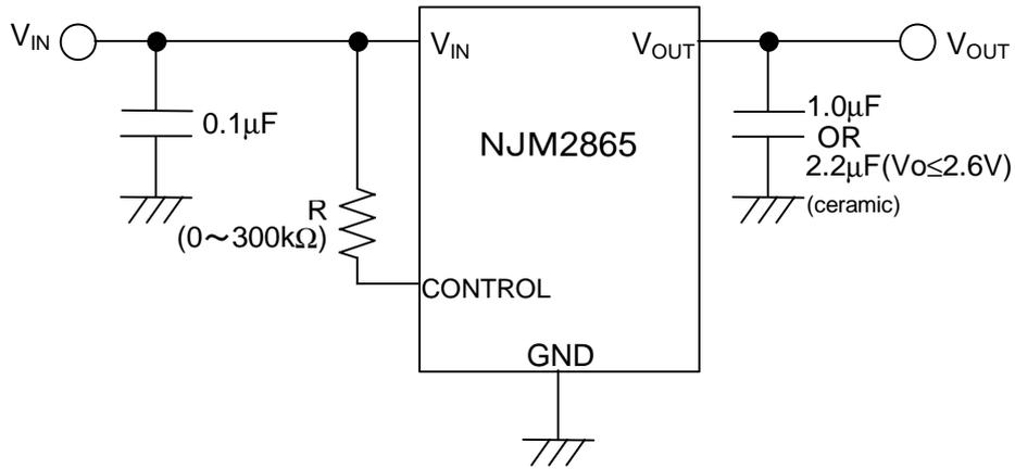
Connect control terminal to  $V_{IN}$  terminal
