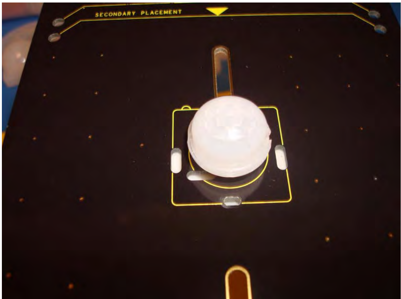
Figure 3. NCL-9(26) Lens and PIR Sensor Installed on the ZMOTION Development Board
