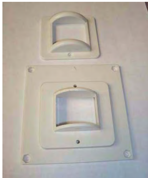
Figure 8. Flat 0.9" Lens Holder (Cap and Base)
