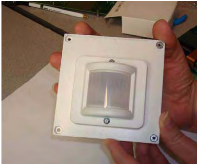
Figure 10. Assembled Flat 0.9" Lens Holder and Flat Lens
