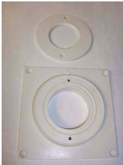
Figure 5. Circular 0.77" Lens Holder (Cap and Base)
