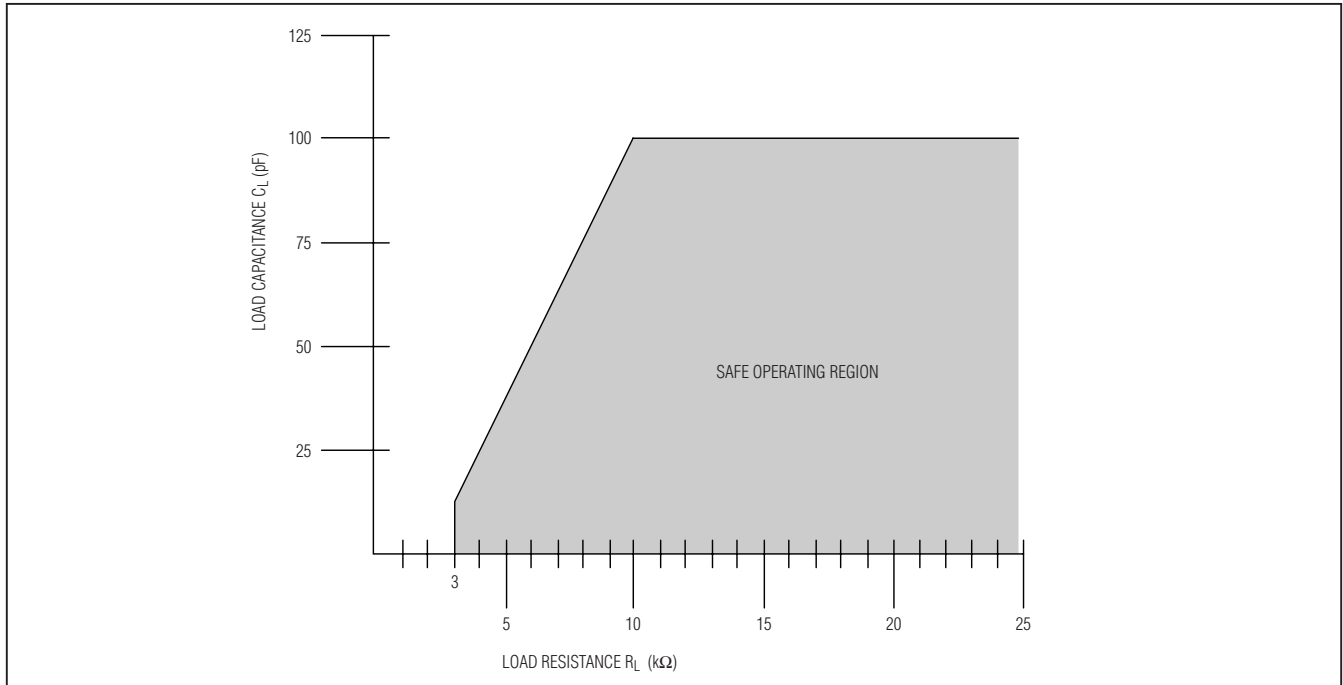
Figure 3. Load-Impedance Operating Region
