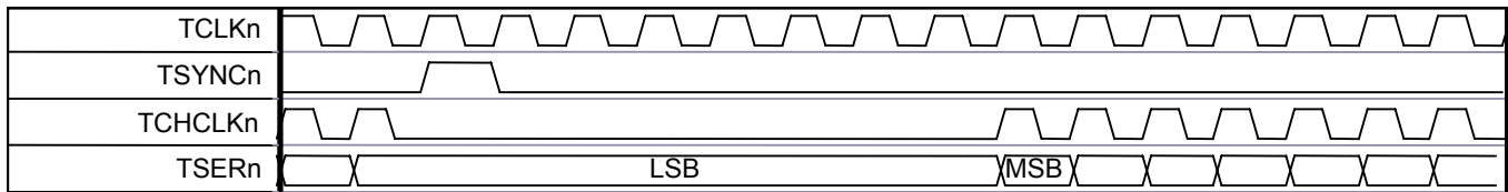
Figure 11-31. E1 Transmit-Side TCHCLKn Gapped Mode During Channel 1
