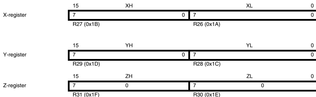
Figure 5-3. The X-, Y-, and Z-registers
