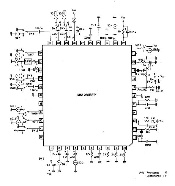
(Note) SWs 1 through 12 should be connected as conditioned in this circuit diagram unless they are otherwise specified in the measuring methods. SG1 and SG2 are both 1.0 VP-P 100% white Y signals, and SG4 is 280 mVP-P chroma burst signal source synchronizing with SG1.
