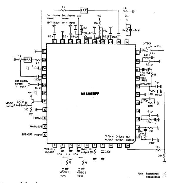
\*Input to pins (3), (3) and (3) should be provided at sufficiently low impedance.
