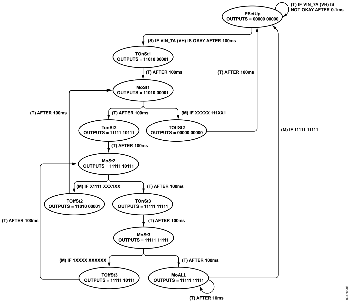
Figure 8. Power Monitor and Sequencing Control Strategy State Machine Diagram
