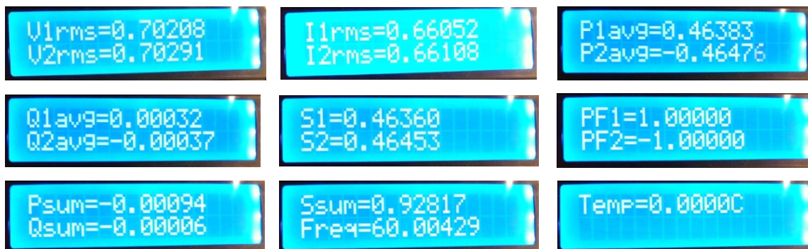
Figure 9. Standalone Power Meter Measurements
