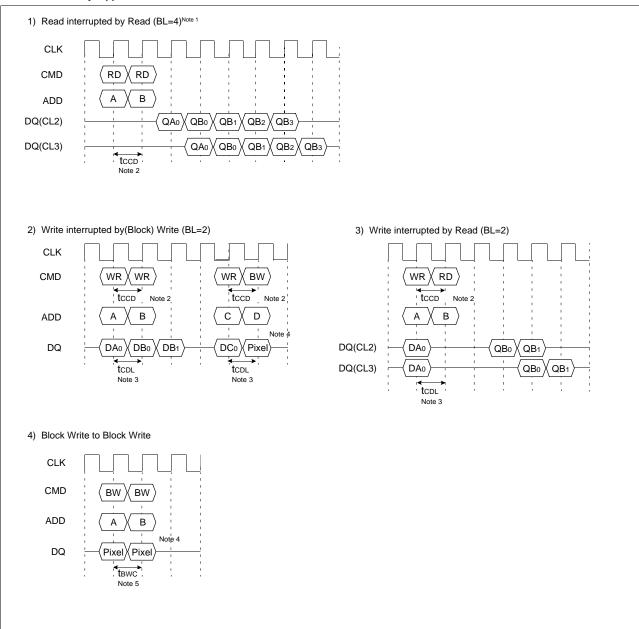
\*Note: 1. By "Interrupt", It is possible to stop burst read/write by external command before the end of burst.
