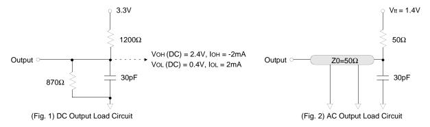
Note: 1. The VDD condition of KM4132G512A-5/C/6 is 3.135V~3.6V.
