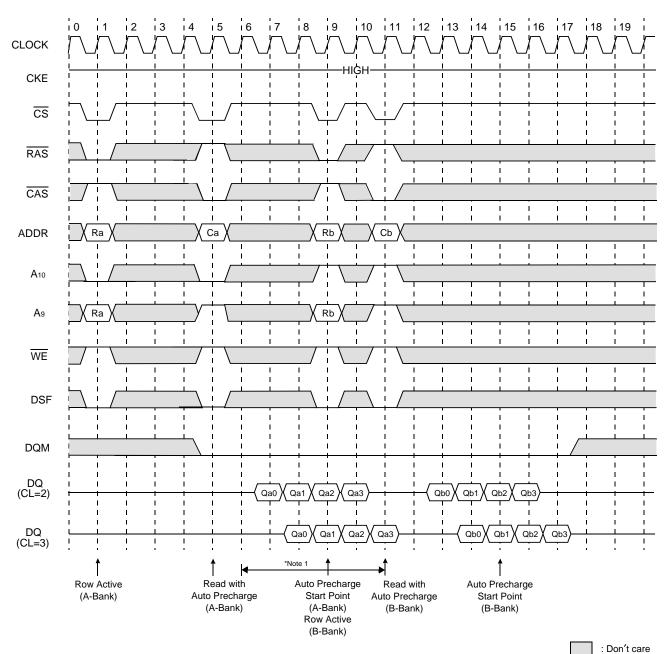
\*Note: 1. Any command to A-bank is not allowed in this period. tRP is determined from at auto precharge start point
