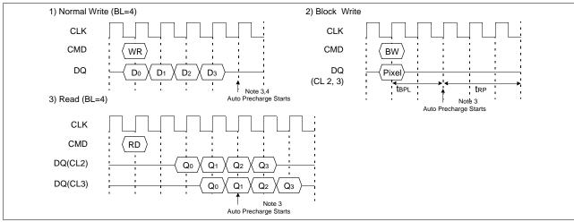
\*Note: 1. tBPL: Block write data-in to PRE command delay
