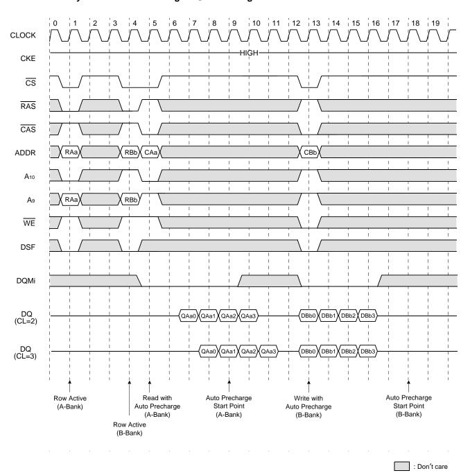
\*Note: 1. tRCD should be controlled to meet minimum tRAS before internal precharge start.
