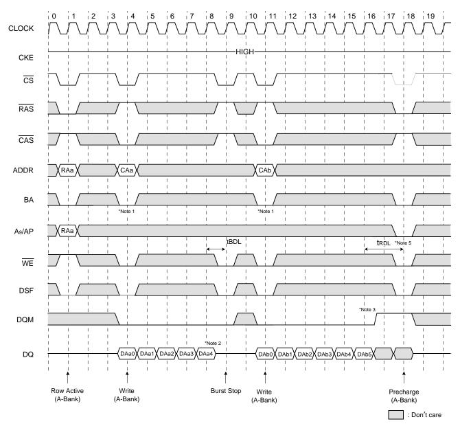
\*Note: 1. At full page mode, burst is wrap-around at the end of burst. So auto precharge is impossible.
