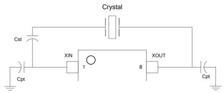
CST - Series Capacitor, used to lower circuit load to match crystal load. Raises frequency offset. This can be eliminated by using a crystal with a Cload of equal or greater value than the oscillator.
