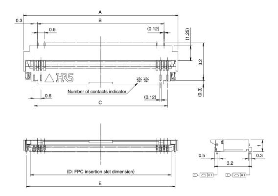
Notes  $\boxed{1}$  The coplanarity of each terminal lead within specified dimension is  $\pm$  0.1 mm.
