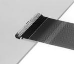
3 Rotate down the actuator until firmly closed. It is critical that the inserted FPC is not moved and remains fully inserted.
