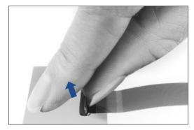
2 Fully insert the FPC in the connector parallel to mounting surface, with the exposed conductive traces facing down.
