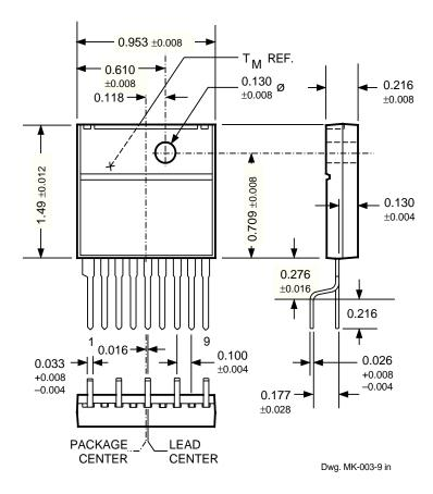
$\label{eq:NOTE:exact body and lead configuration at vendor's option within limits shown. \\$
