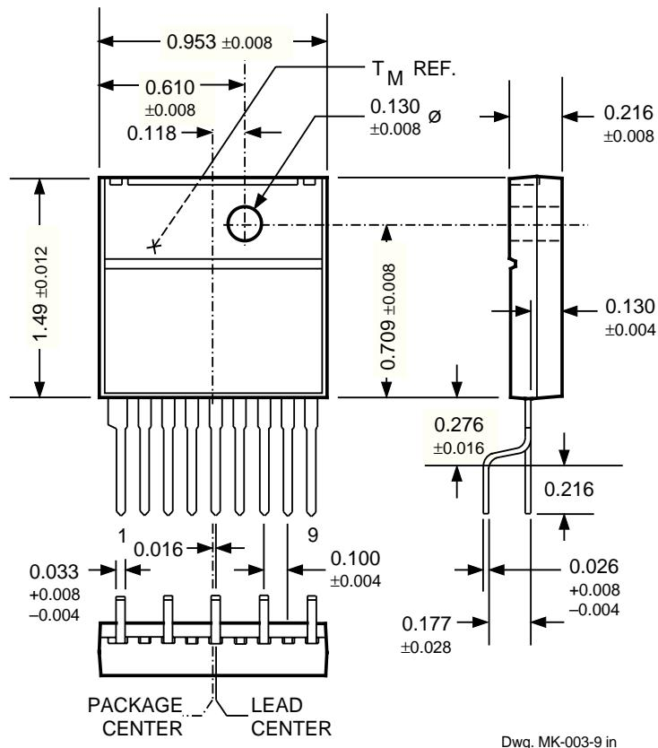
NOTE: Exact body and lead configuration at vendor's option within limits shown.
