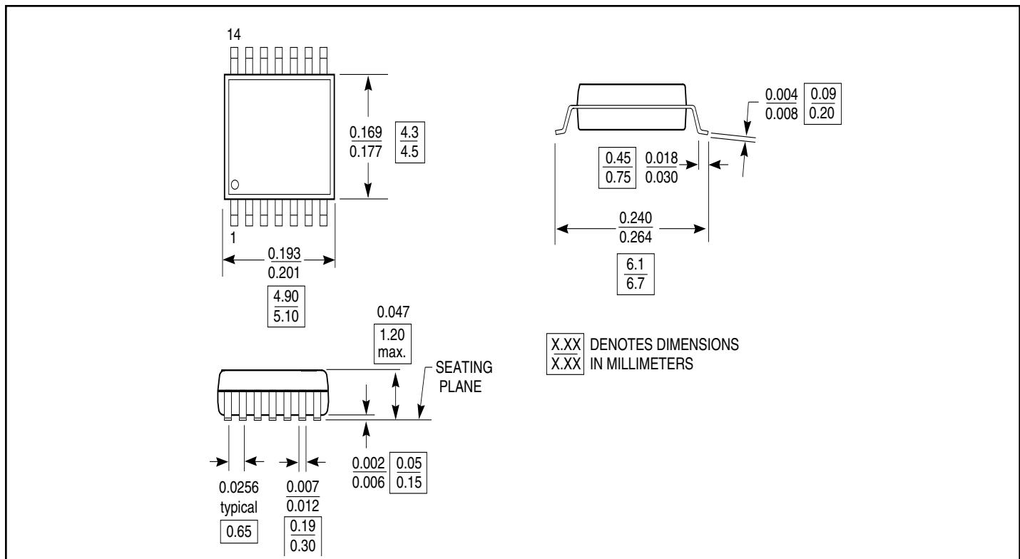
**Packaging Mechanical: 14-Pin SOIC (W)**
