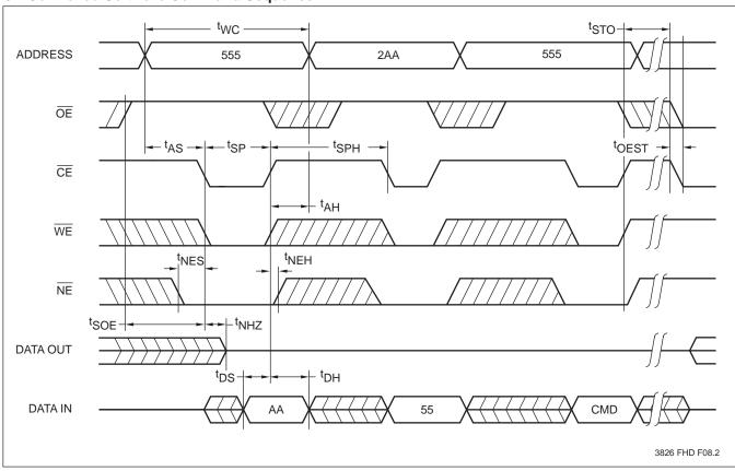
**Note:** (6) The Store Pulse Width (t<sub>SP</sub>) is a minimum time that  $\overline{NE}$ ,  $\overline{WE}$  and  $\overline{CE}$  must be LOW simultaneously.
