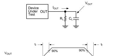
**Functional Characteristics Test Circuit**
