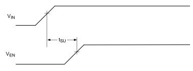
Figure 1c. Input-to-Enable Setup Timing
