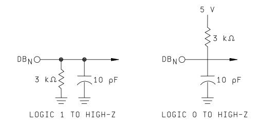
FIGURE 7. Load circuit for output float delay test.
