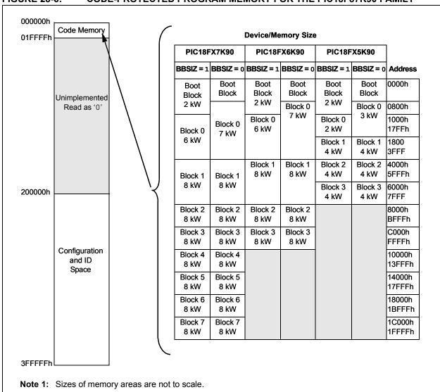
2: Boot block size is determined by the BBSIZ0 bit (CONFIG4L<4>).
