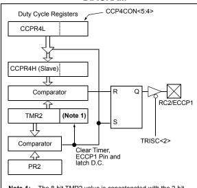
Note 1: The 8-bit TMR2 value is concatenated with the 2-bit internal Q clock, or 2 bits of the prescaler, to create the 10-bit time base.
