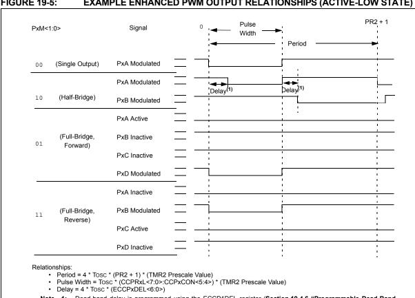
Note 1: Dead-band delay is programmed using the ECCP1DEL register (Section 19.4.6 "Programmable Dead-Band Delay Mode").
