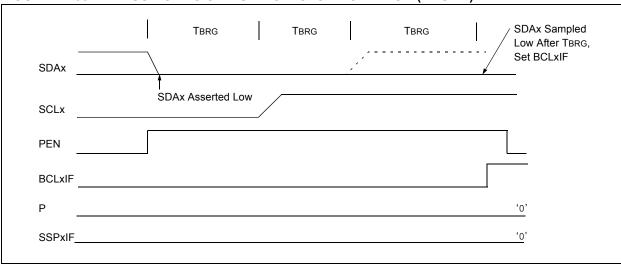
FIGURE 21-34: BUS COLLISION DURING A STOP CONDITION (CASE 2)
