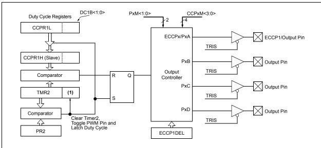
Note 1: The 8-bit TMR2 register is concatenated with the 2-bit internal Q clock, or 2 bits of the prescaler to create the 10-bit time base.
