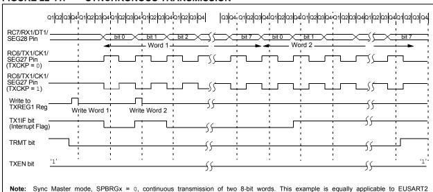
FIGURE 22-12: SYNCHRONOUS TRANSMISSION (THROUGH TXEN)
