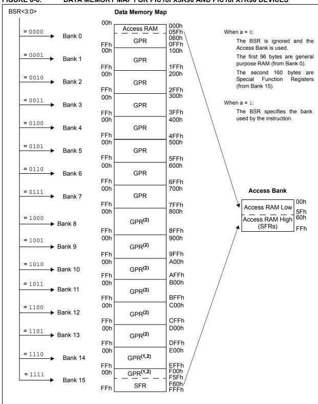
FIGURE 6-6: DATA MEMORY MAP FOR PIC18FX5K90 AND PIC18FX7K90 DEVICES
