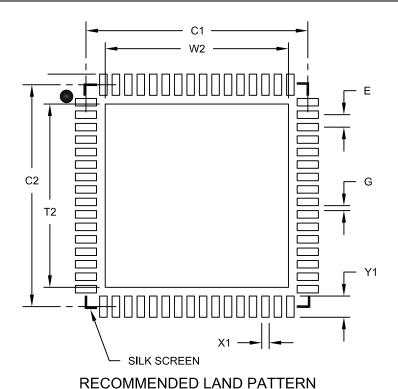
Units **MILLIMETERS** MIN MOM MAX **Dimension Limits** Contact Pitch 0.50 BSC Ε Optional Center Pad Width W2 7.35 Optional Center Pad Length 7.35 T2 Contact Pad Spacing C1 8.90 Contact Pad Spacing C2 8.90 Contact Pad Width (X64) Χ1 0.30 Contact Pad Length (X64) Υ1 0.85 Distance Between Pads G 0.20
