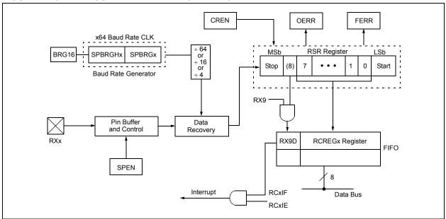
FIGURE 22-7: ASYNCHRONOUS RECEPTION
