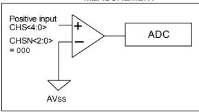
In the Single Channel Measurement mode, the negative input is connected to AVSS by clearing the CHSN bits (ADCON1<2:0>).
