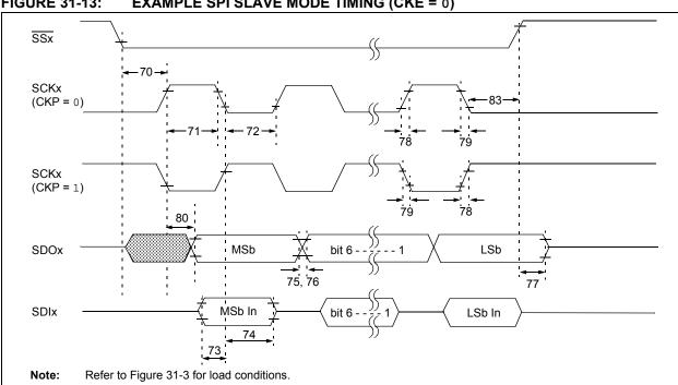
FIGURE 31-13: **EXAMPLE SPI SLAVE MODE TIMING (CKE = 0)**
