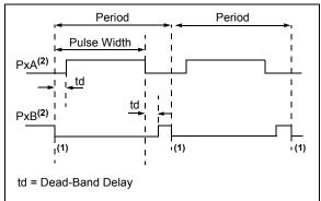
Note 1: At this time, the TMR2 register is equal to the PR2 register.
