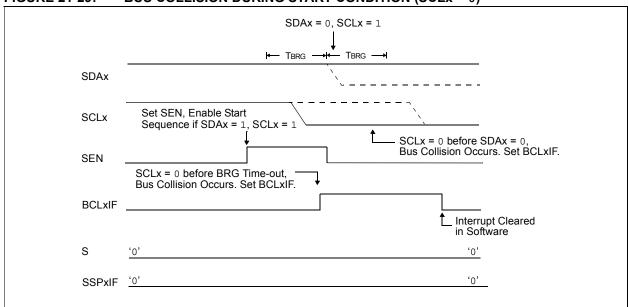
FIGURE 21-30: BRG RESET DUE TO SDAX ARBITRATION DURING START CONDITION
