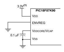
Note 1: These are typical operating voltages. For the full operating ranges of VDD and VDDCORE, see Section 31.2 DC Characteristics.
