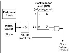
Clock failure is tested for on the falling edge of the sample clock. If a sample clock falling edge occurs while CM is still set, a clock failure has been detected (Figure 28-5). This causes the following:
