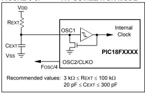
The RCIO Oscillator mode (Figure 3-4) functions like the RC mode, except that the OSC2 pin becomes an additional general purpose I/O pin. The I/O pin becomes bit 6 of PORTA (RA6).
