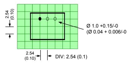
Dimensions are typical values: mm (inch) General Tolerance:  $\pm 0.25 (\pm 0.01)$ Pin Tolerance:  $\pm 0.1 (\pm 0.004)$
