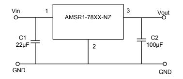
C1: A low ESR capacitor is required to keep the noise of the converter to a minimum.
