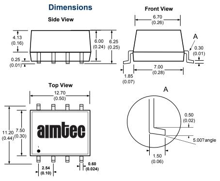
All dimensions are in mm (inch) All Pins are on a 2.54mm (0.10inch) pitch with tolerance of ±0.25mm (0.01inch)
