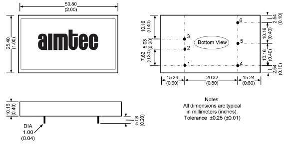
Pin Diameter: 1.0±0.05mm (0.04±0.002 inches) Pin pitch tolerance: ±0.35mm (±0.014 inches)
