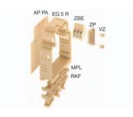
Larger housings are easily assembled: the intermediate plate (ZP) and the connection spigot (VZ) enable 2 or more housings to be mechanically joined together. The ZP joins together the housing frames at the bottom of the frame. The locking combination foot or the mounting plate allows the housing to be mounted on the rail or directly.
