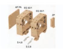
Larger housings are easily assembled: the inter-mediate plate (ZP) allows 2 or more housings to be mechanically joined together. The ZP joins together the housing frames in the area of clamping yoke unit.
