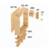
Larger housing are easily assembled: the intermediate plate (ZP) and the connection spigot (VZ) enable 2 or more housing to be mechanically joined together. The ZP joins together the housing frames in the area of the clamping yoke unit and the VZ the housing frames at the bottom of the frame. The fixing in combination foot or the mounting plate allows the housing to be mounted on the rail or directly.
