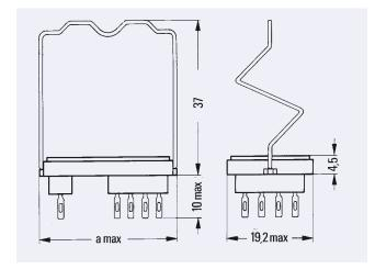
with hold-down spring for cradle relay W
