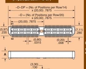
Specify **LEAD** STYLE = Gold Flash from on Signal Pins and chart Ground Plane, Matte Tin on tails
