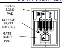
DIE SIZE: 12.6X16.9 mils (320x430  $\mu$ m) DIE THICKNESS: 3 mils (75  $\mu$ m) BONDING PADS: 3.3X2.4 mils (85x60  $\mu$ m)
