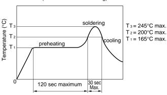
VPS (Vapor Phase Soldering)
