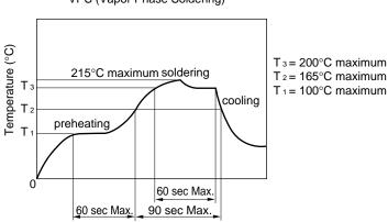
Note: 1.Temperature profiles show the temperature of PC board surface.
