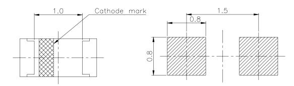
**Note:** The tolerances unless mentioned is  $\pm 0.1$ , Unit = mm
