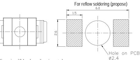
Note : Tolerances dimension ±0.1 unless otherwise noted Unit : mm
