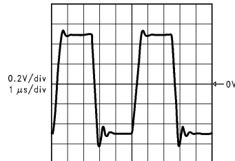
Large Signal Step Response V_S = \pm 1.35V, A_V = +1, Z_L = 10\text{ k}\Omega \parallel 20\text{ pF}, V_{IN} = 1\text{ V}_{PP}
