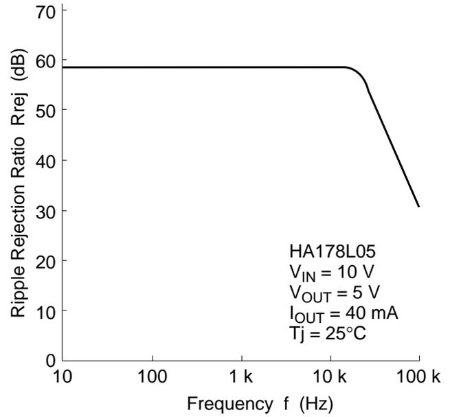
Ripple Rejection Ratio vs. Frequency (3)
