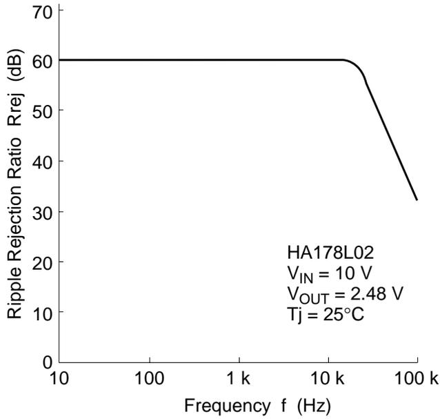
Ripple Rejection Ratio vs. Frequency (2)
