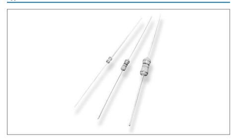
The resistive element comprises a thin film of nickel-chrome alloy evaporated onto a high thermal conductivity ceramic element. Metal end caps are force fitted to the element prior to spiralling to value. Tinned copper lead wires are welded to the end caps and the components are then coated. One coat of phenolic resin is followed by three coats of epoxy resin. All resistors are tested for value and tolerance.
