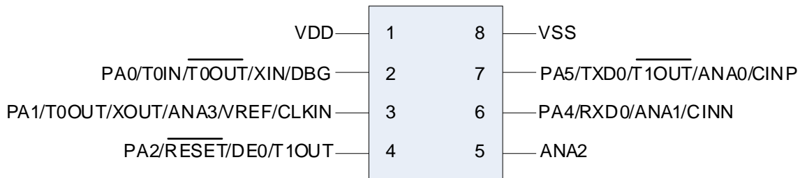
Figure 2. 8-Pin SOIC Package Diagram – Z8FS040xSB20EG
