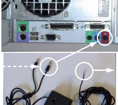
Connect the R11 jack "in parallel" with Tip/Ring of modem
