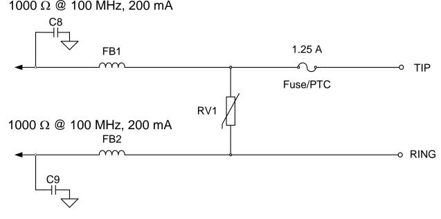
Figure 26. Circuits that Pass All UL1950 Overvoltage Tests
