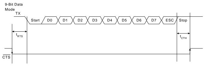
UART Timing for Modem Transmit Path (9N1 Mode with 9th Bit Escape)
