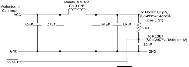
Figure 29. Modem Module V<sub>CC</sub> and RESET Filter
