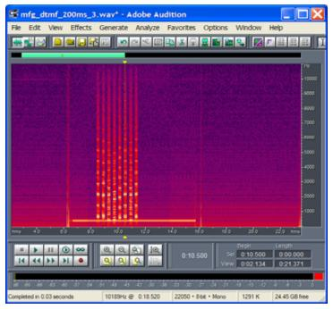
Figure 71. Defective DTMF
