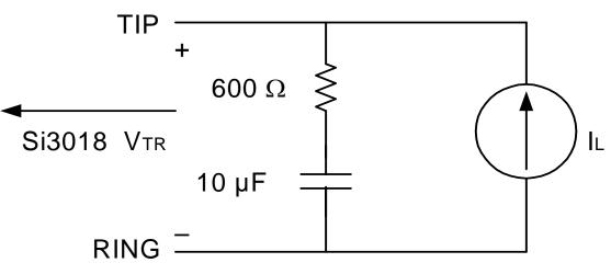
Figure 10. Phone Line Termination Circuit
