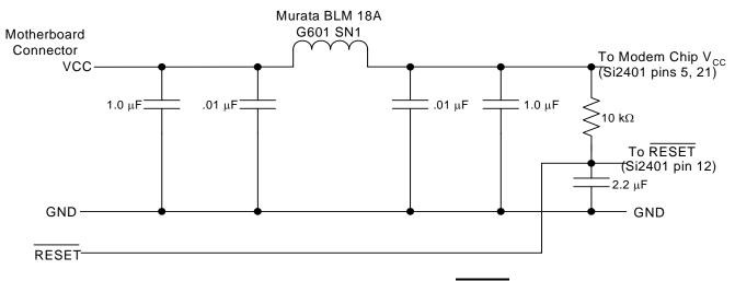
Figure 44. Modem Module V<sub>CC</sub> and RESET Filter
