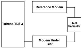
Figure 24. Bell 103–V.34 Modem Functional Test Connection
