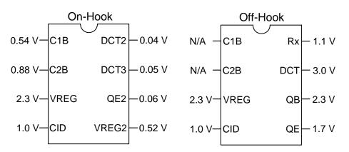
Voltages measured with respect to IGND (Si3008 pin 9)
