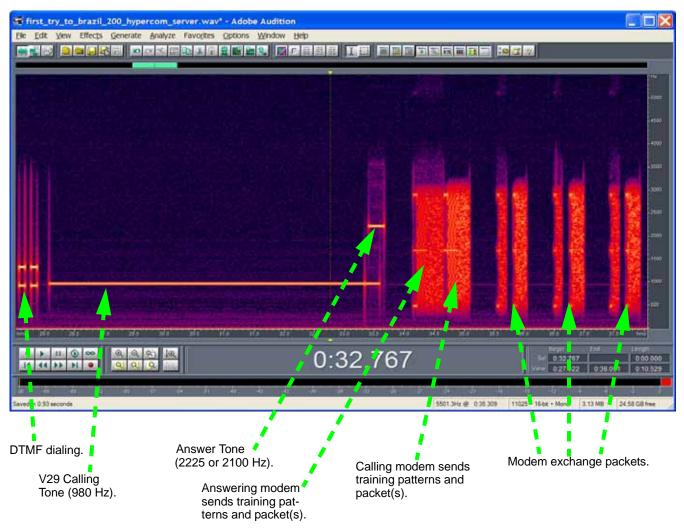
Figure 68. Appearance of V29FastPOS Protocol
