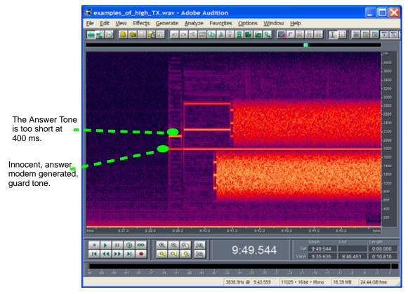
Figure 70. Example of EPOS Server Misbehavior
