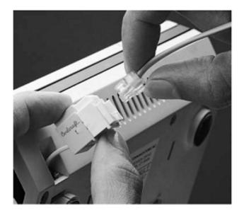
Eliminating common mode EMI from telephone lines, handset cords, and LANs can be done quickly and easily with these plug-in filter modules.
