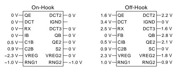
Voltages measured with respect to IGND (Si3018 pin 15)
