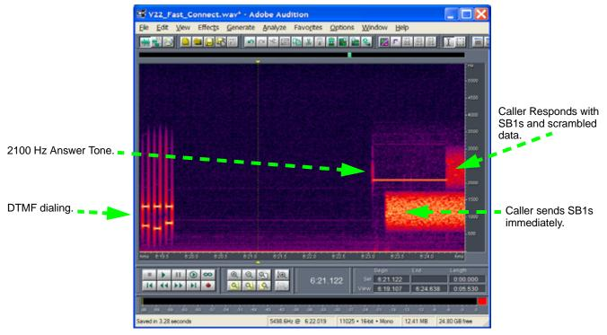
Figure 67. Appearance of V.22 Fast Connect Protocols
