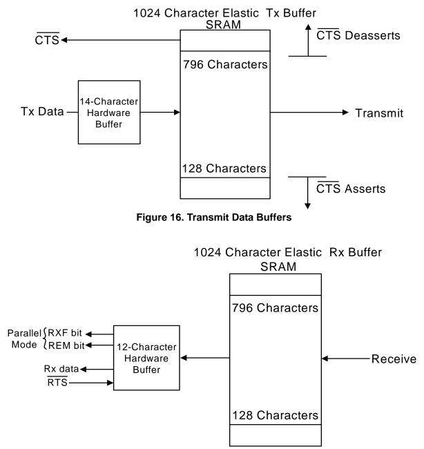
Figure 17. Receive Data Buffers
