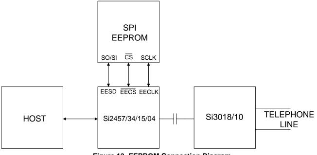
Figure 13. EEPROM Connection Diagram
