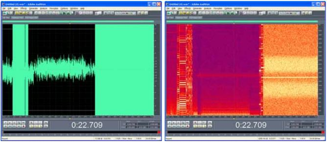
Figure 62. Recording Made at Excessive Level
