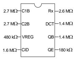
Resistance measured with power and phone line removed Figure 50. Si3008 In-Circuit Resistance to IGND (Si3008 Pin 9)
