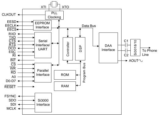
Figure 9. Si2493/57/34/15/04 Functional Block Diagram
