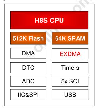
The **EXDMA** unit becomes the TFT-LCD controller, requiring only 5% of CPU bandwidth for example when refreshing a WQVGA TFT-LCD panel at 60Hz, moving graphic RGB data from external RAM into the TFT panel. Plenty of CPU bandwidth remains to drive the remainder of the application and to create medium animation.
