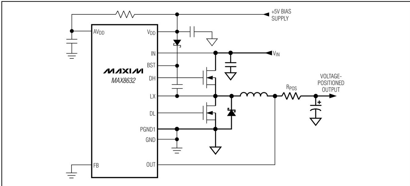
Figure 9. Voltage-Positioned Output
