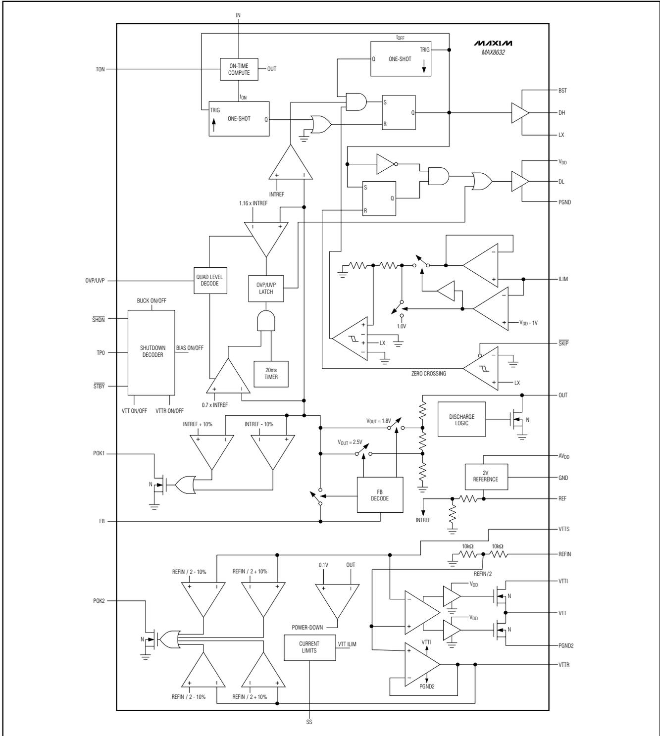
Figure 1. Functional Diagram
