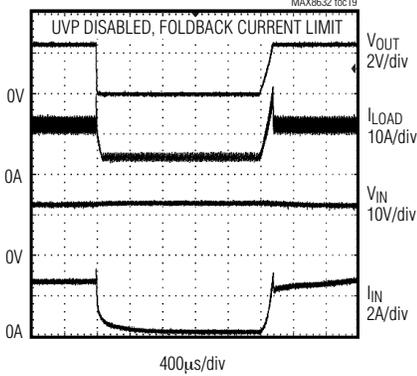
SHORT CIRCUIT AND RECOVERY OF  $V_{DDQ}$
