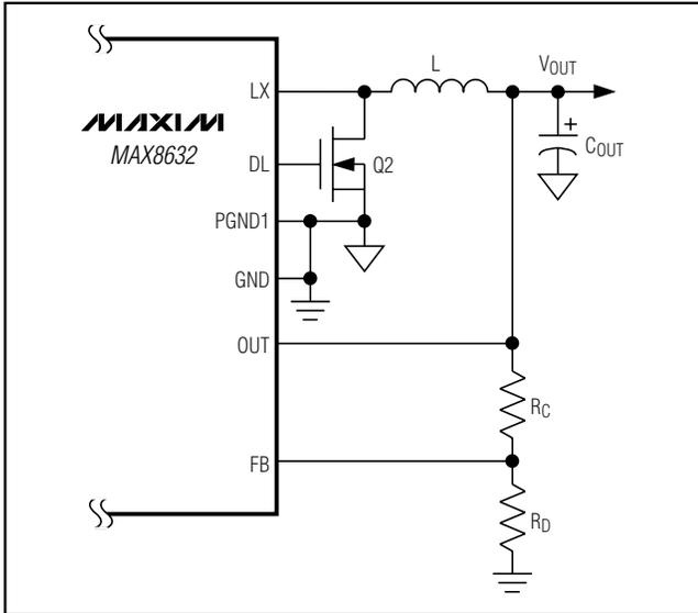
Figure 6. Setting  $V_{OUT}$  with a Resistive Voltage-Divider
