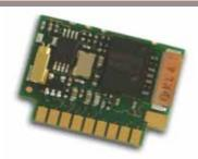
This miniature module enables full duplex Bluetooth® data or audio transmissions over 20m.
