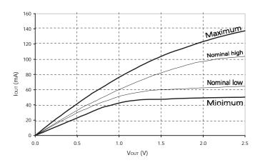
Figure 14: Full Drive Pull-Up Characteristics
