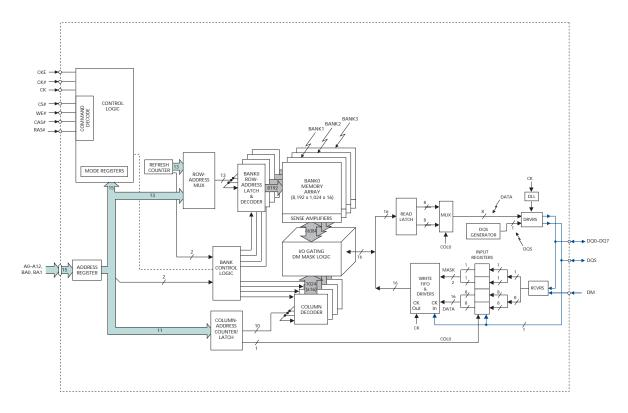
Figure 5: 32 Meg x 16 Functional Block Diagram
