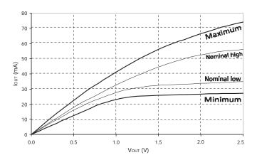
Figure 16: Reduced Drive Pull-Up Characteristics
