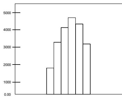
This histogram represents the typical peak-to-peak noise (including quantization noise) associated with the ADS-937.
